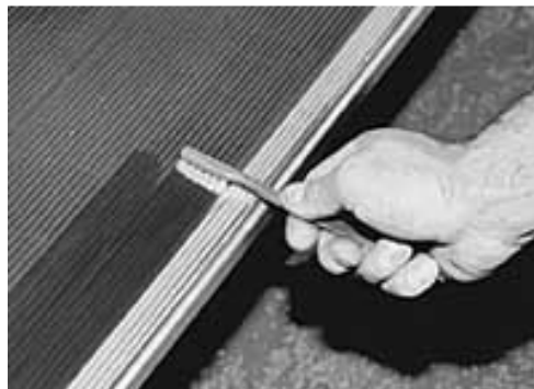
A stiff brush is the best way to clean the grooves of this classic era running board.
