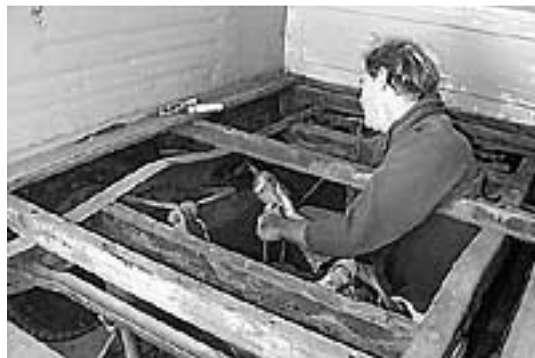
Figure 2 Using a wire wheel and drill to clean your car's chassis is safer than sand blasting.
