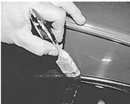
A natural bristle paint brush, cut down, is great for cleaning in grooves and door cracks.
